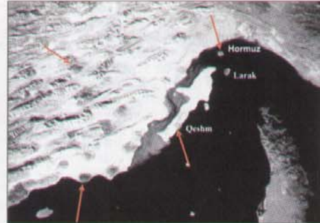
Fig. 5 Zagros chains, salt domes on- and off-shore are characterized by dark subcircular structures on this Landsat image
