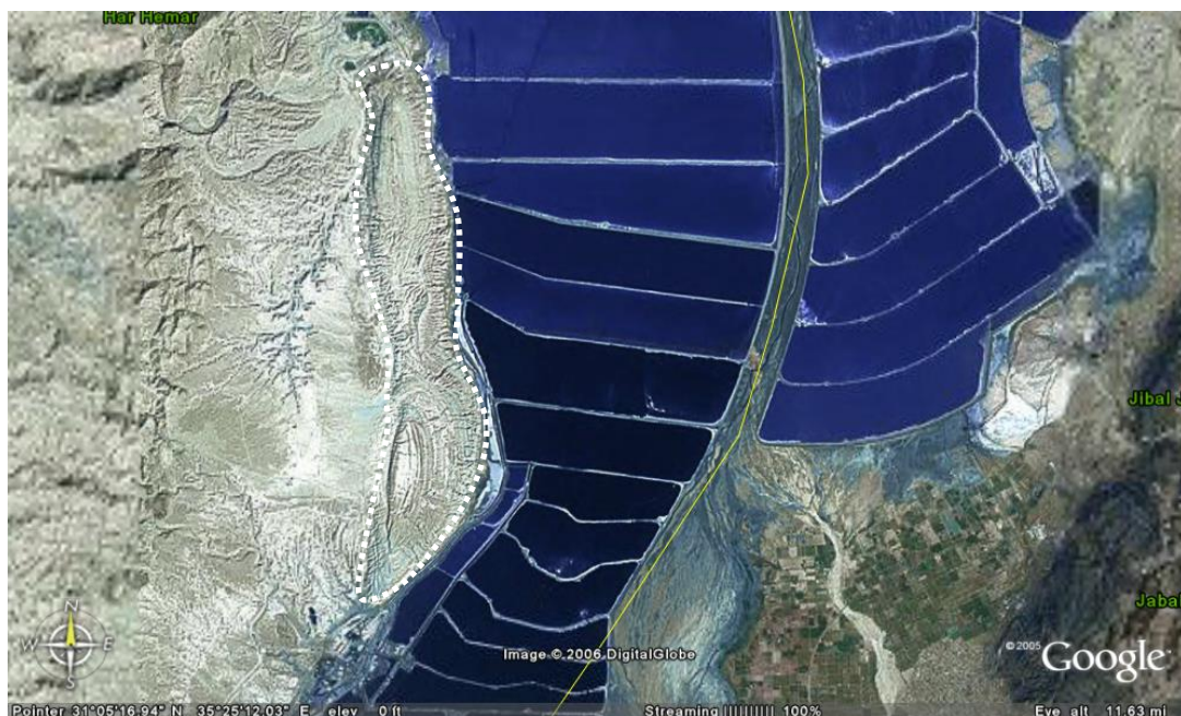
Figure 9: Evaporation pans in Israel (left) and Jordan (right) south of the Dead Sea. The Mount Sdom salt structure is marked by a dotted line. Steep layers suggest a view at a cross section of a salt lake.
