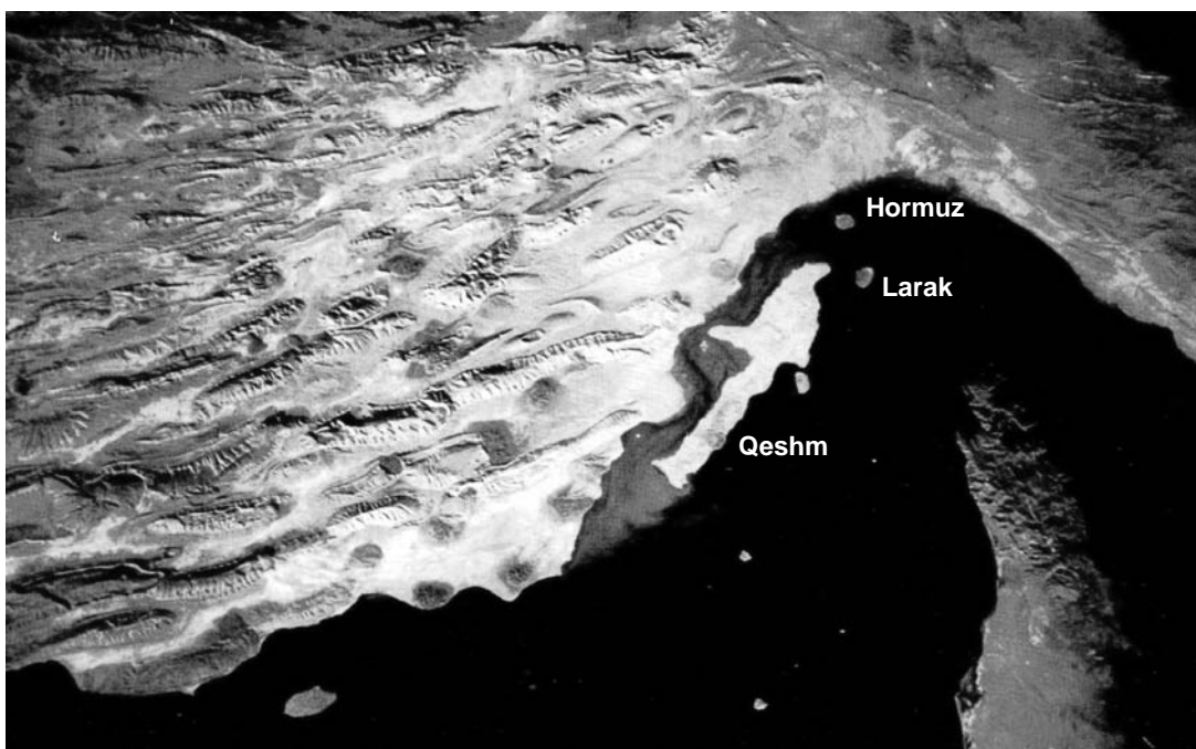
Figure 5: Zagros chains, salt domes on- and off-shore are characterized by dark subcircular structures on this Landsat image.
